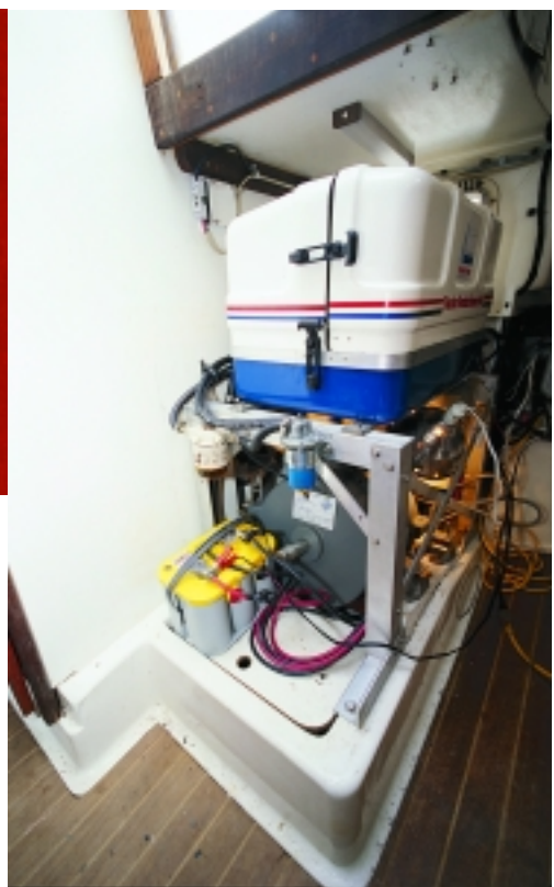
Left: An exploded view of the Electric Wheel. Above: Bud Virts's Hunter 33 with Electric Wheel and generator installation.
